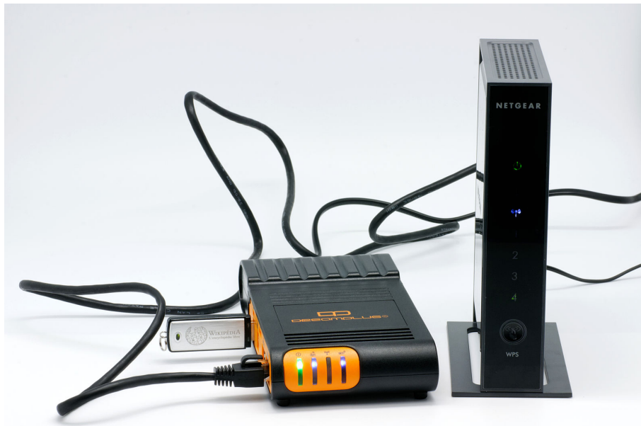
Figure 1: The hardware used in the Afripedia project consisting of a plug computer, a wireless router as well as a USB drive containing a copy of the French Wikipedia [15]
